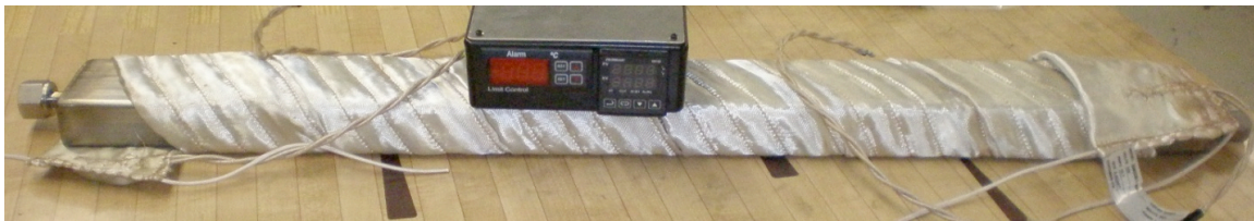
Figure 2. Test section, heater, and control box.
