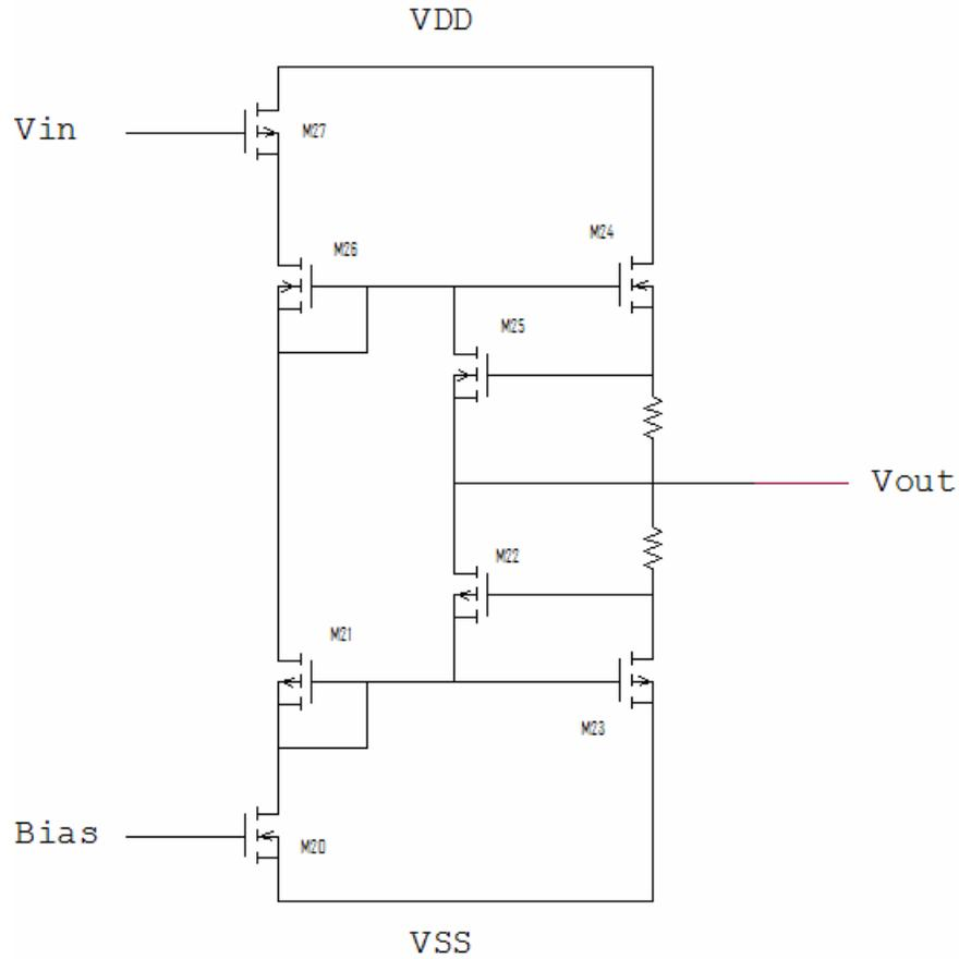
Figure 3: AB output with current limiting scheme
