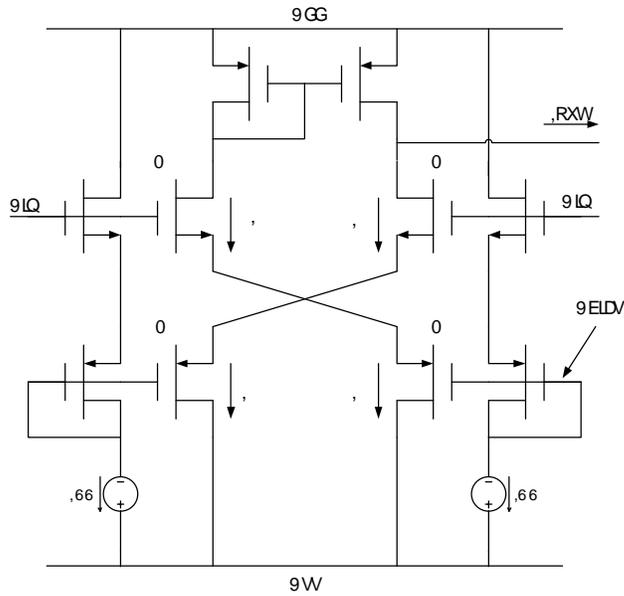
Figure B-1: Source Cross-Coupled Differential Amplifier
