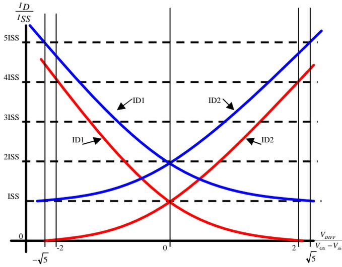
Figure B-3: Normalized drain current transfer characteristics for source cross-coupled and bias cross-coupled differential amplifier. The dashed line is the source cross-coupled; the solid line is the bias cross-coupled.
