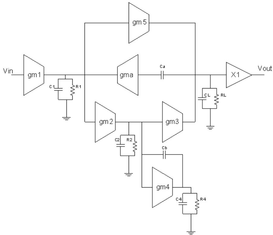
Figure 1: Three-Stage, Dual Path Amplifier Topology
