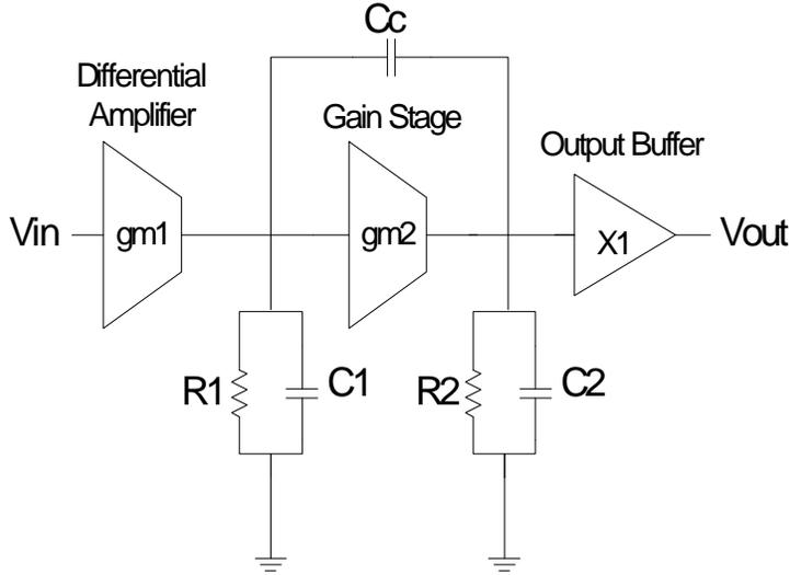
Figure A-1: 2-Stage Amplifier Topology
