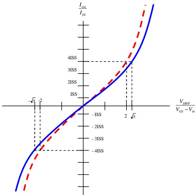
Figure B-4. Normalized output current transfer characteristics for source cross-coupled and bias cross-coupled differential amplifier. The dashed line is the source cross-coupled; the solid line is the bias cross-coupled.
