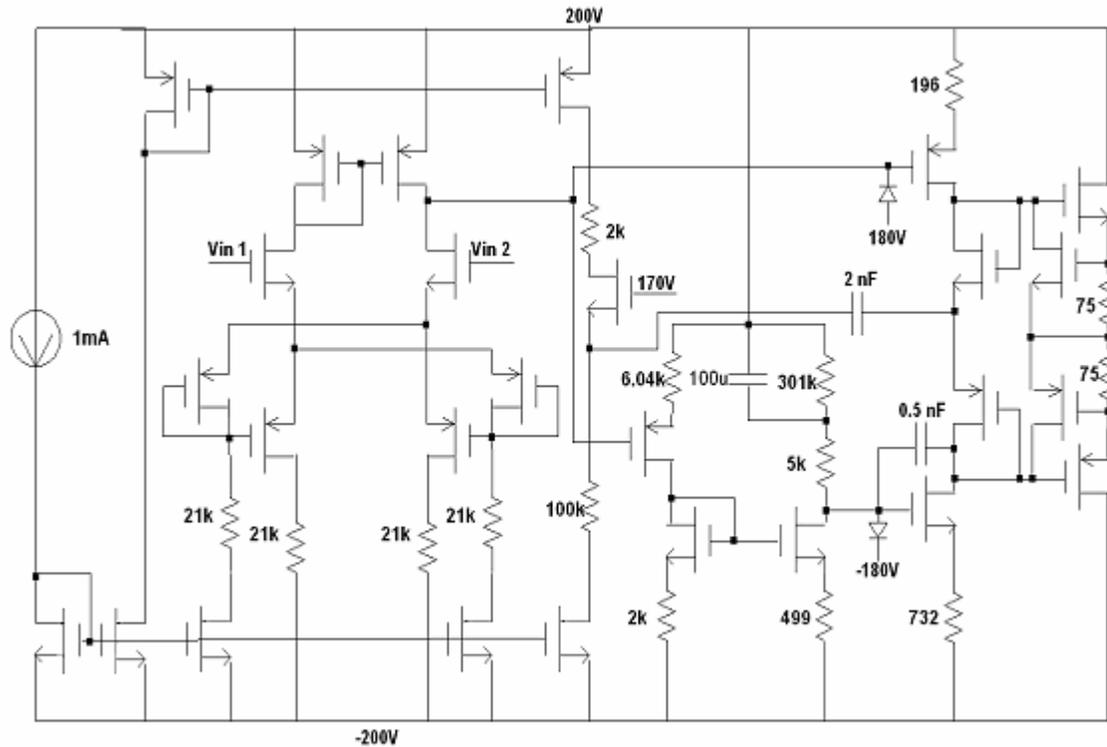
Figure 4: Full Circuit Schematic
