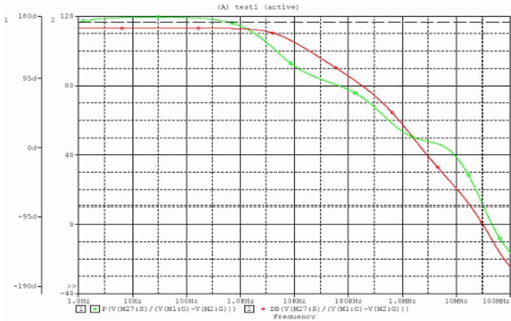
Figure 9: Uncompensated Gain Simulations
