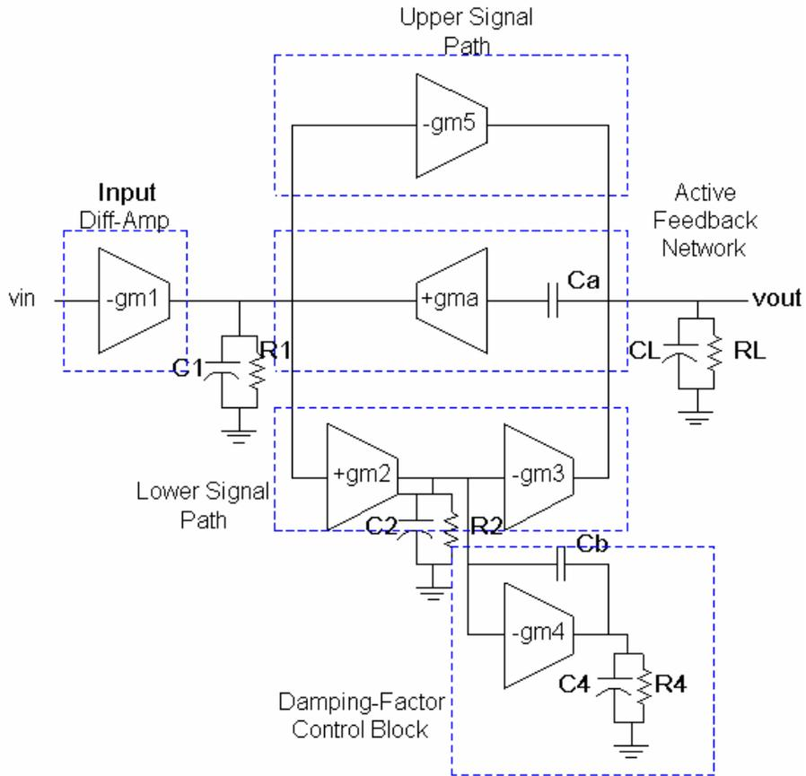
Figure A-2: 3 Stage, Dual Path Amplifier
